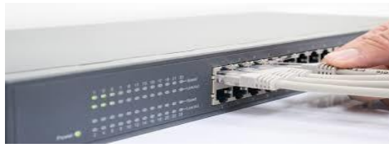
Figure 22: Network Switch with Cable Connections
