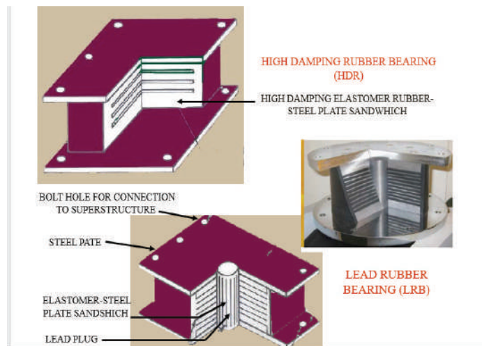
Fig. 23: Base Isolation Devices
