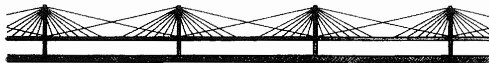
(b) Long cables from a pylon head to an adjacent pylon at the deck level
