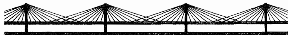
(c) Cable stays coming from both adjacent pylons to support the central part of each span.
